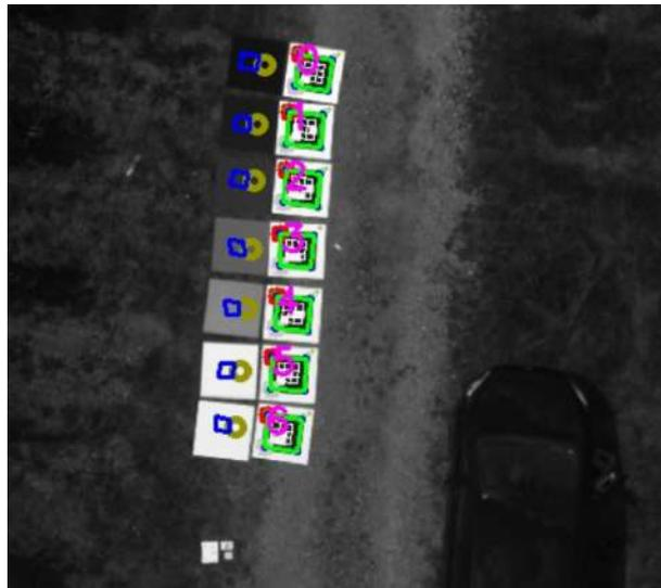
Figure 11 An aerial image augmented with the detected reference panels. The numbers (violet) indicate the identified marker ID, while the areas enclosed by blue lines are used for the extraction of the DNs.
