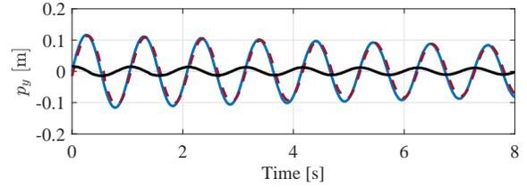
Fig. 5. Experimental validation of the developed KF. Blue line: Real y-position, Red line: Estimated y-position, Black line: Estimated velocity.
