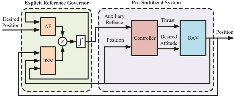
Fig. 2. Proposed ERG-based scheme for geofence applications.
