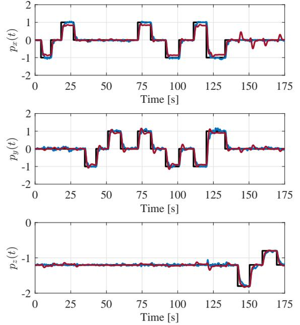
Fig. 6. Validation of the approximated linear model for the AR Drone. Black line: Desired position, Blue line: Real position, Red line: Position obtained via identified linear model.
